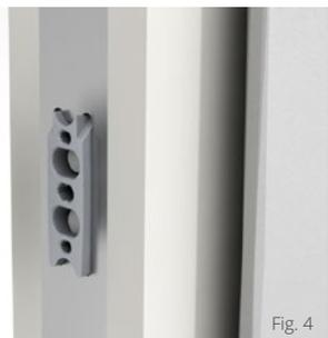
In the event of emergency, if you cannot remove the door handle on the inside of the hinge, prise open the door, applying serious force around the handle area (see Fig. 3, p. 12). With 1 kN of force, the safety clip on the latch will yield and the door will open (see Fig. 4, p. 12).
