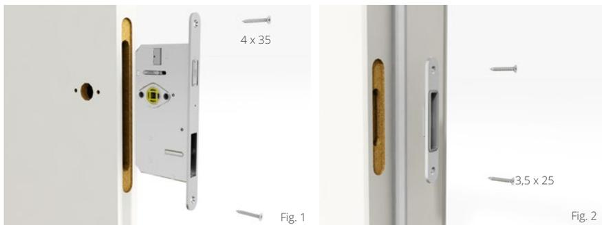
1. Insert the lock into the recess intended for it and fasten with two countersunk screws, 4.5 x 35 (included) as shown in Fig. 1. Use suitable tools to tighten the screws hand-tight.
